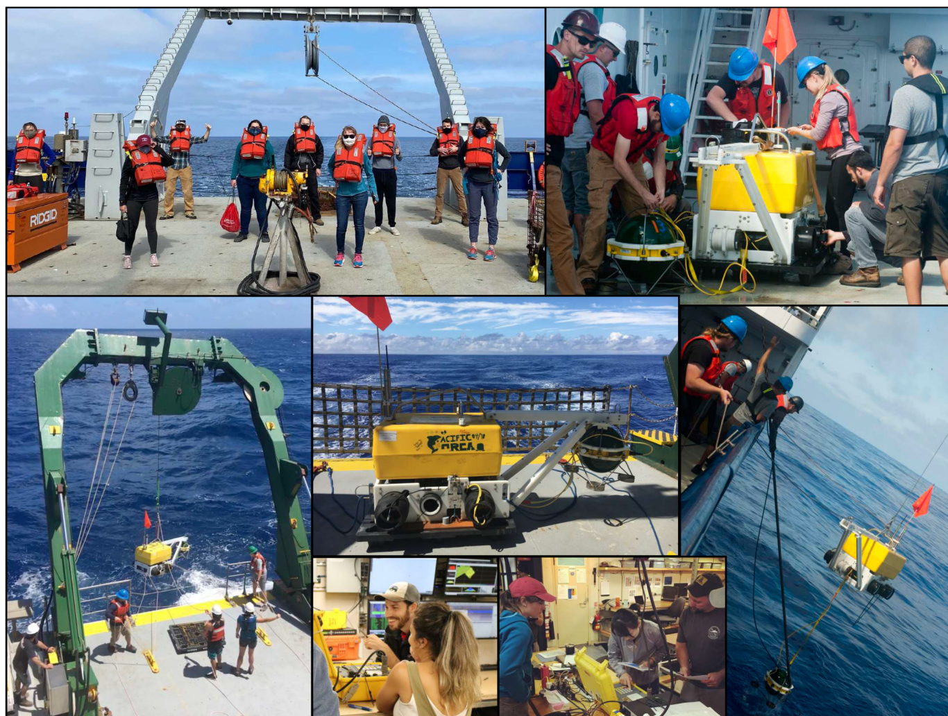
Figure 2. Fieldwork photos from deployment and recovery of both arrays. Center figure: Scripps Institution of Oceanography (SIO) OBS on back deck of R/V Kilo Moana prior to Old ORCA deployment. Clockwise from top left: Science party conducts fire drill on back deck of R/V Roger Revelle during Old ORCA recovery; disassembly of Old ORCA instrument following recovery; tag lines being affixed to sensor ball during Old ORCA recovery; students and SIO OBS tech communicating with Old ORCA instrument during postdeployment acoustic survey using EdgeTech 8011M deck box connected to hull-mounted 12 kHz transducer; student and PI issuing burn command to release instrument during Old ORCA recovery; young ORCA instrument deployment from A-frame of R/V Kilo Moana for Young Orca array. Photo credits: H. Janiszewski, E. Nathan, and Z. Eilon. The color version of this figure is available only in the electronic edition.
